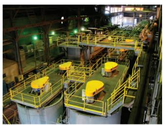
The new 50 m<sup>3</sup> WEMCO Smart flotation cells.
